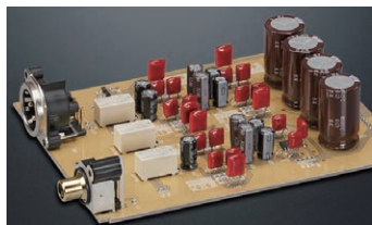
Glass cloth fluorocarbon resin PCB with Direct Balanced Filter circuitry
