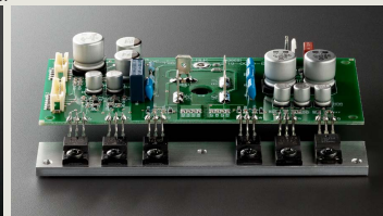
Dedicated power supply for signal input section
