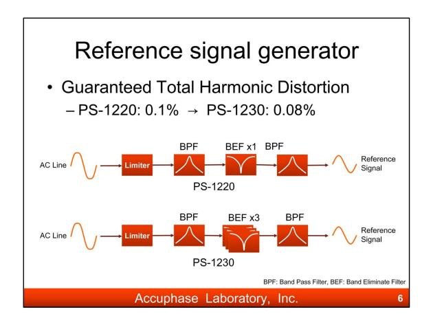
Reference signal generator is the circuit which eliminates the noise and distortion components in AC line signal with filters and generates the reference signal for waveform shaping.
