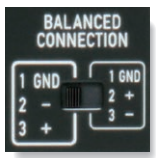
Phase selector switch
